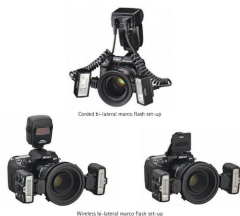
Fig. 9: Unidirectional Flashes Mounted In A Bi-Lateral Configuration (Twin Flash)
